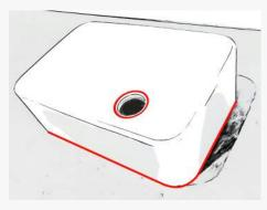
2. Once basin is in position, apply all along the outside edge and along the waste hole.
