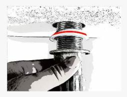
4. Apply to rubber thread at the bottom of the waste and finish by ONLY hand tightening. Over tightening may cause the basin to crack.
