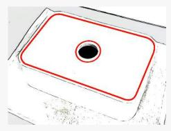
1. Place basin upside down onto a towel and apply near the edge and near the waste hole.
